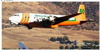
The Erickson Aero Tanker 60, a DC-7 first built in 1958 for Eastern Air Lines, likely retired in October, while Erickson's converted MD-87s first operated by SAS are in demand as fire-fighting tankers.
